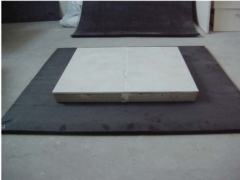
Figure 5-3: 40mm concrete plinth on 15mm Thermotec Impact Foam sample.
