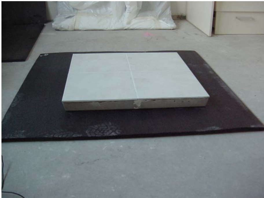
Figure 5-2: 40mm concrete plinth on 10mm Thermotec Impact Foam sample.
