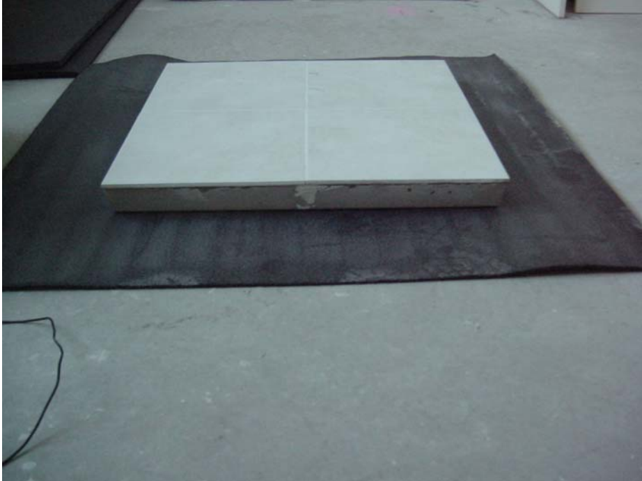
Figure 5-1: 40mm concrete plinth on 5mm Thermotec Impact Foam sample.
