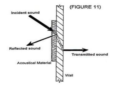
Barriers are usually HARD surfaces that REFLECT sound leading to Echo. Rw 13dB @ 50MM per ISO 717-1
