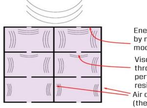
Energy dissipation by membrane mode (loss factor) Viscous loss through perforation (flow resistance) Air cavity effect (thermo viscous boundary layers)
