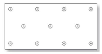
Suggested Layout of fasteners on a 1200 x 2400mm sheet.
