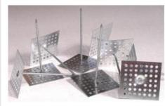
Insul anchors have 12 ga (2.7mm) diameter mild steel spindles with a corrosion resistant coating. The perforated base plate is 50mm square and is made of galvanized steel. Standard lengths range from 25mm through to 240mm and are packed 1,000 pieces per carton up to 64mm; 500 pieces per carton for longer sizes.
